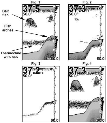
These figures show results of different sensitivity levels on the same location. Fig. 1: Sensitivity at 87 percent, determined by Auto Sensitivity. Typical of full auto mode. Fig. 2: Sensitivity set at 50 percent. Fig. 3: Sensitivity set at 20 percent. Fig. 4: Sensitivity set at 100 percent.
